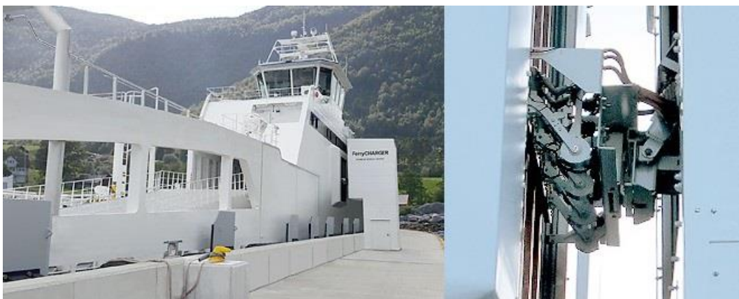
Figur 11 Vertikal pantograflader for ferger, ref Stemman, [2]
